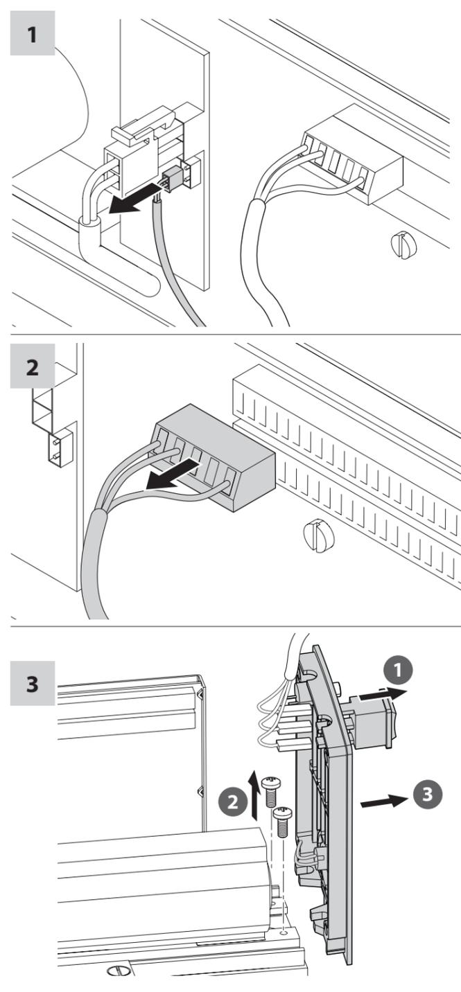
**Reinstall the new reset switch, the programme switch and the new side panel**
