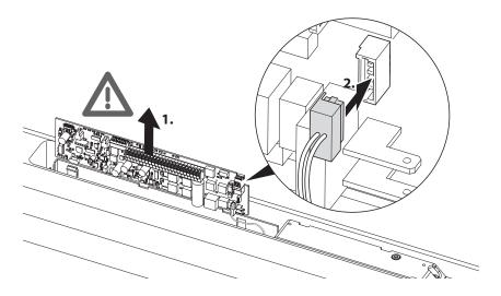
▶ Connect the 24-V cable of the motor gear unit.
