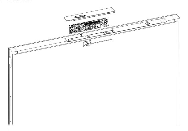
Hook in using your finger or a tool (notch) and carefully lift out the control circuit board
