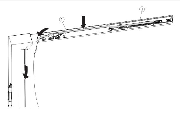
Route cable (1) along the motor gear unit (arrow) to the control circuit board (2).
