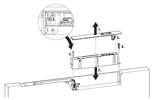
► Connect the rotary encoder cable of the motor gear unit.
